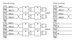
Marking indicates output signal polarity when the circuit is active. Polarity reverses when the circuit is not active. Wire notification appliances accordingly. Notification appliance polarity shown in active state.
